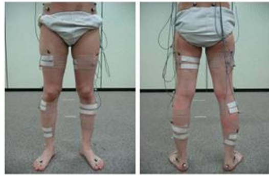
Fig. 1. Subjects who had reflective markers and EMG electrodes for the gait motion experiment.
